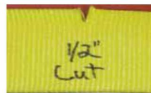
Actual Break: 14,000 pounds Loss from BL Break: 49% Loss from Min. Break: 42%
