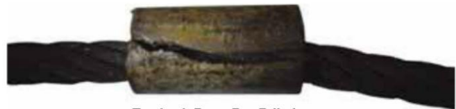
Turnback Eye - Eye Failed
