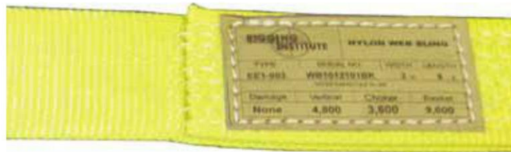
Vertical Rated Capacity 4,800 pounds Minimum Break (Min.) Strength: 24,000 pounds Actual Break-Base Line (BL): 27,510 pounds
