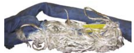
This shows a sling failure due to stitching that punctured core yarns.
